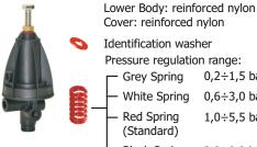
Cover: reinforced nylon Identification washer Pressure regulation range: 0,2÷1,5 bar Grey Spring White Spring 0,6÷3,0 bar Red Spring 1,0÷5,5 bar (Standard)
